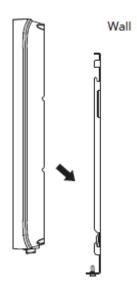
5. Secure the BioStation 3 to the bracket with the BioStation 3 Fixing Screw.
