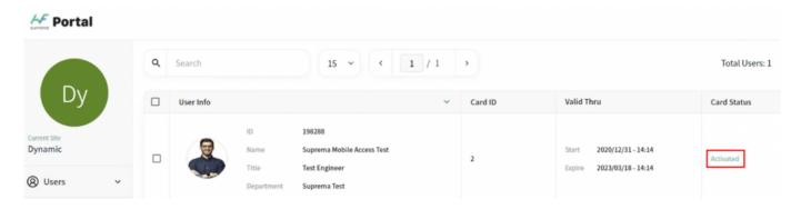
**Step 8.** Turn on the phone's NFC or BLE function and authenticate the Mobile Access Card to the device registered in **Step 3**. You can check the user authentication log in BioStar  $2 \rightarrow$  Monitoring.
