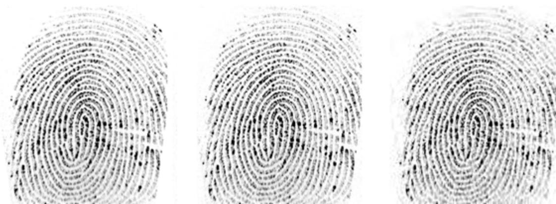
(a) Original gray image (b) Compressed image by WSQ (5:1) (c) Compressed image by WSQ (15:1)
