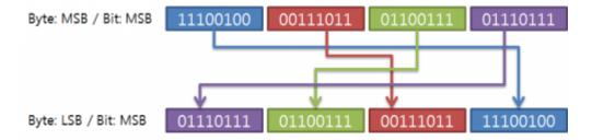
Lastly, change the byte and bit orders to LSB. The resulting number is 668,788,462, which is 00100111 11011100 11100110 11101110 in the binary number. If you read the number read in the LSB byte order and the MSB bit order backward, the two numbers are the same.
