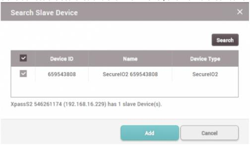
One master device can connect up to 31 devices, but up to 8 fingerprint devices are able to be connectable through RS485. We recommend minimum number of RS485 connected fingerprint devices considering the number of users and connected devices. This is because it can lead to slow matching speed depending on the device which is used for "Master" device.
