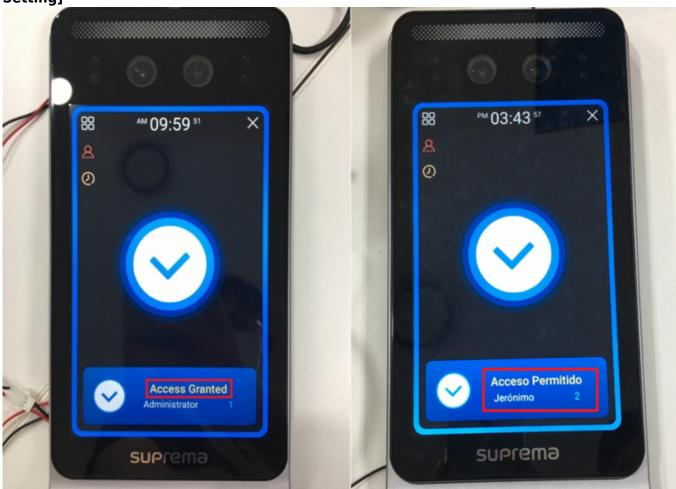
It is possible to customize languages, or to change the message displayed on the device by configuring the device's resource file. Follow the steps below to change the texts displayed on the device (Facestation F2).
