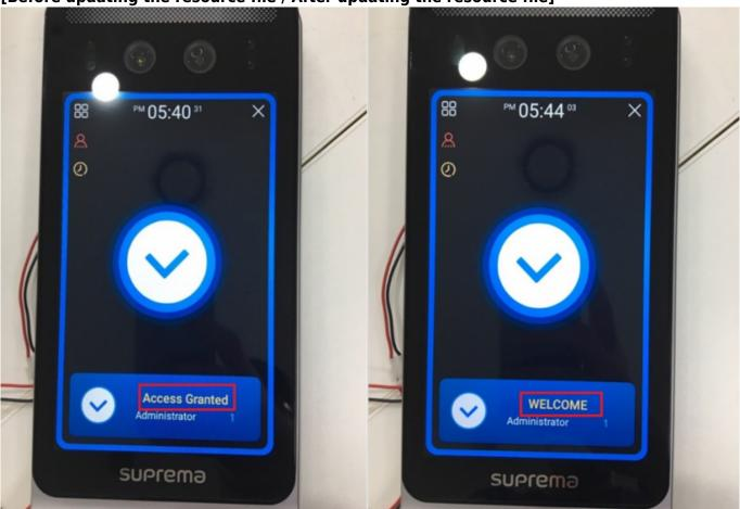
It is possible to customize languages, or to change the message displayed on the device by configuring the device's resource file. Follow the steps below to change the texts displayed on the device (Facestation F2).
