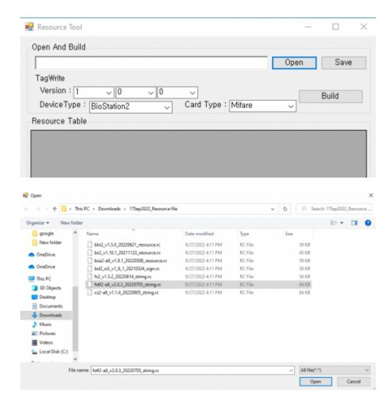
5. Fill out the information at **TagWrite** (Firmware Version, Device Type, Card Type). Note that the **DeviceType** must match to read resources at BioStar 2.
