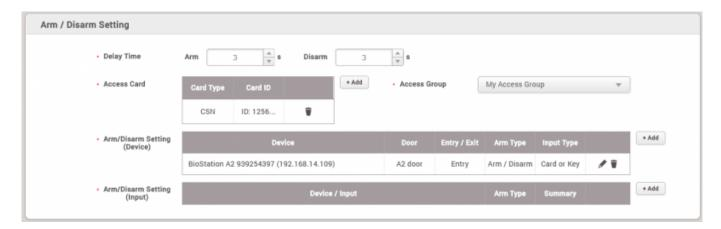
12. Configure the input to detect intrusion by clicking **+Add**. The door sensor is also used to detect intrusion.
