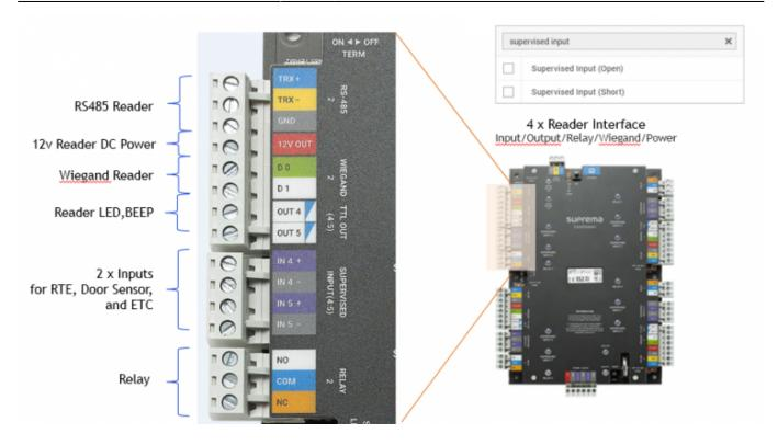
The device's input is a supervised input. This means that the device can sense if the input has tampered just like the DM-20.
