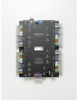
Since it is a centralized controller, CoreStation does not have a reading capability unlike other edge devices and its role is to control the slave and wiegand devices that are connected to the device. It has 4 relays, 4 wiegand inputs, and 5 RS485 channels where you can connect slave devices.
