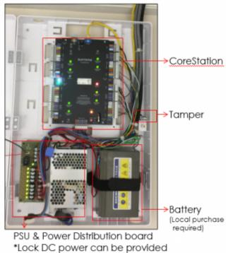
CoreStation also comes with an optional enclosure which includes power supply unit and the power distribution board.
