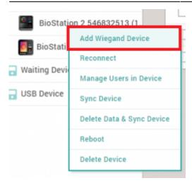
You cannot use the device as a slave device and use Wiegand output at the same time.
