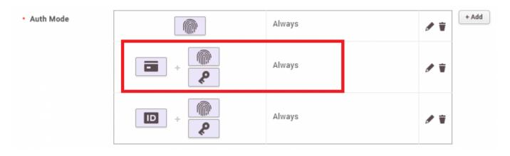
5-2. Once you succeed in card authentication on a 3rd-party device, the Wiegand input signal will be sent to the Suprema reader. After that, the Suprema reader requests you to scan fingerprints on it. If you succeeded in scanning fingerprints on the Suprema reader, the below event will happen as if "Card + Fingerprint" authentication is generated in one device.
