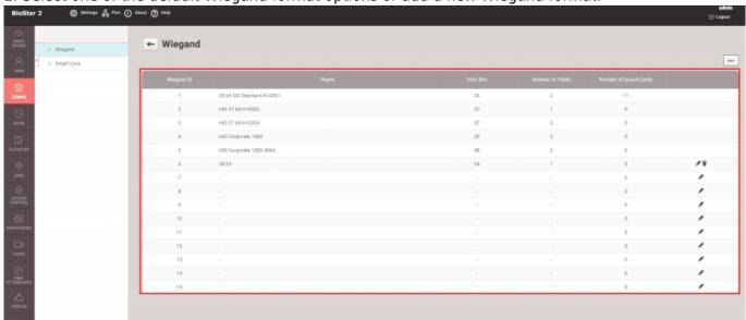
3. Wiegand format can be set by assigning the total bits, ID field, and parity bits. For example, in order to configure 34 bits card format with parity bit checks by half of each even and odd parity check logic, it's necessary to set 'Start Bit' and 'End Bit' for each part.
