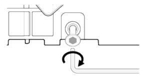
When assembling the product with the bracket, you can use the included bracket fixing screw(Star Shaped) instead of the product fixing screw for enhanced security.
