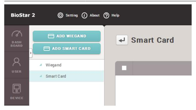
2) Enter the name of the smart card format. There are 4 types of cards supported for the AoC card and the SC card, Mifare, iClass, DESFire, and iClass Seos (added in BioStar 2.6). Select the card that will be used for the smart card.
