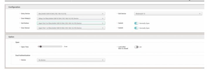
3) If the door sensor is applied, Held Open and Forced Open alarm can be set to use. Click '+Add' button on the left and set to use 'Output' and select the device to make an 'Output' and the relay to send out an output signal. But if you want to make an alert only, you need to set the device which is not used for the door relay or other important output to the 'Device' and its relay to 'Output'. This is because it can be mixed and create an unplanned relay output.
