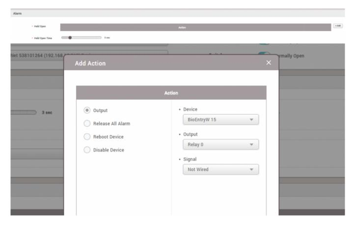
i.e. Held Open Alarm Configuration for the door This configuration will help to generate the Held door open alarmed log once the door opened log is kept more than Held Open Time.
