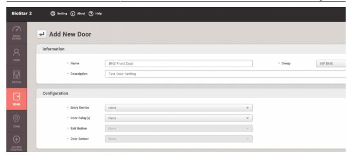
2. Set **Entry Device** and select 'Exit Device' when the door uses two devices for entry and exit. And set 'Door Relay', 'Exit Button', and 'Door Sensor', according to the door situation.
