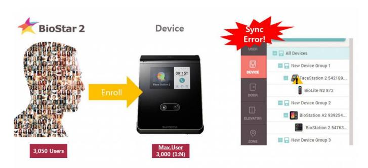
ASync error occurs when data exceeds device capacity.
