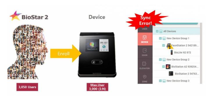
ASync error occurs when data exceeds device capacity.
