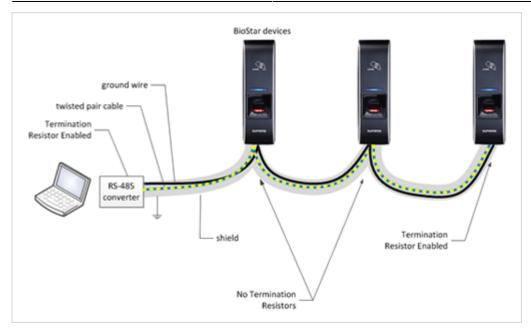
Avoid using long stubs for each node. Long stubs act as transmission lines and should be kept as short as possible if unavoidable.
