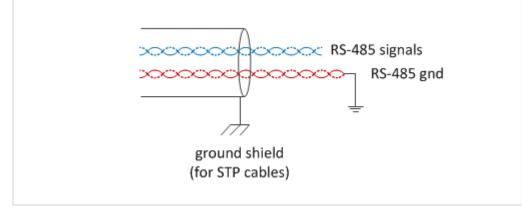
The following restrictions apply to RS485 connections: **BioStar 1** PC Connection: maximum 31 devices Master - Slave Connection : maximum 7 slave devices
