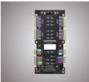
Input Module is a multiple input extension module which can control up to 12 supervised inputs, 2 AUX, 1 temper switch and 2 relays. A total of 31 units can be connected to a master device via an RS485 daisy chain. It allows the use of inputs for interfacing with sensors or door contacts etc., as well as providing a simple 'dry contact' interface for other systems.
