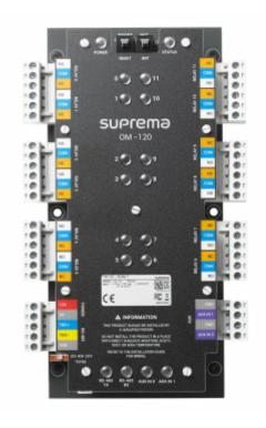
The OM-120 is a 12-relay output control module. When used together with BioStar 2, it is able to control the access to select floors from the elevator.
