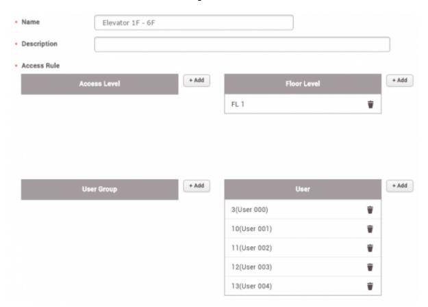
If configured like the image above, the buttons to access the 1st to 6th floor will be initiated for *User 000*, *User 001* and *User 002* when using *Elevator 1*.
