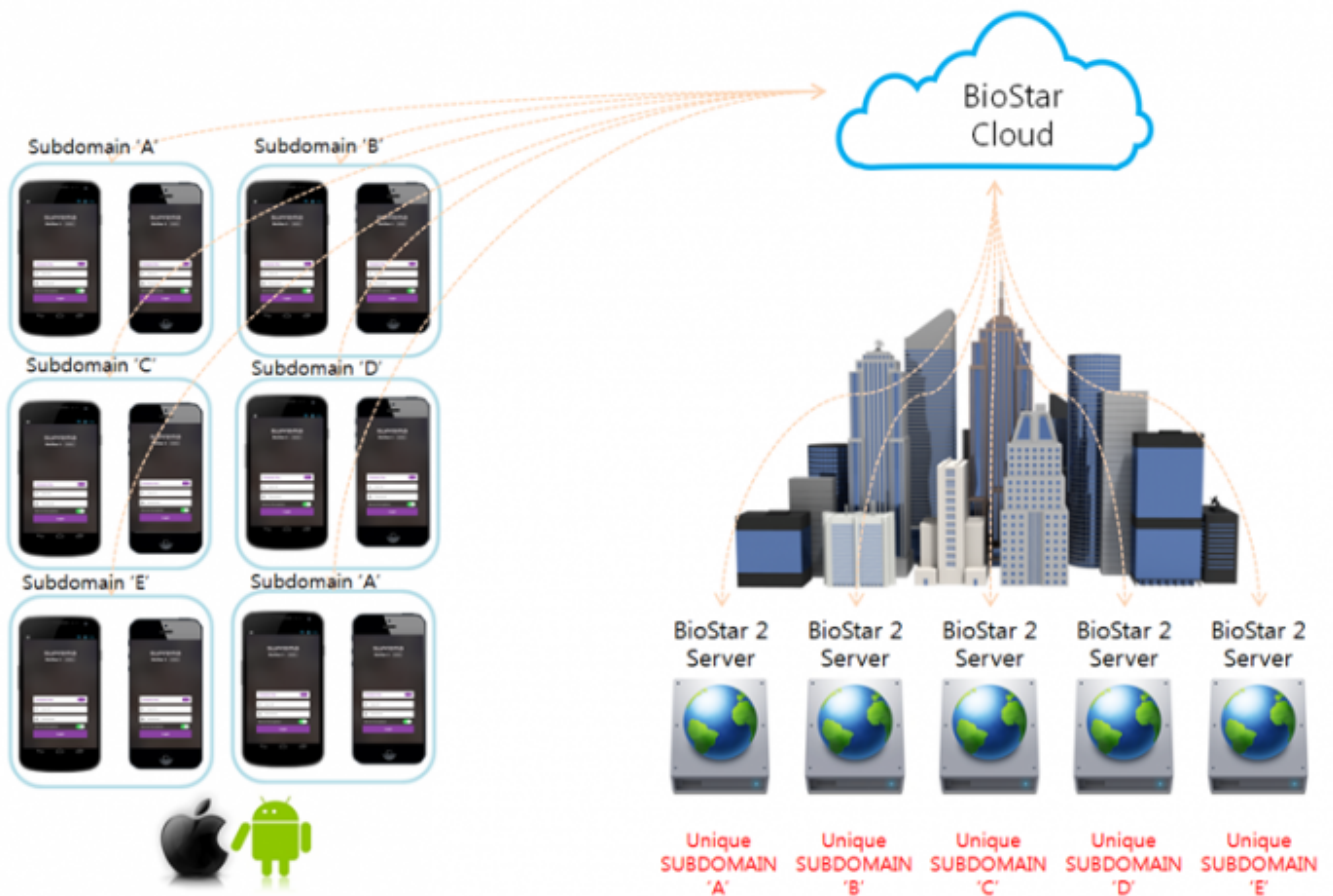
[Overall Architecture of BioStar 2 Mobile]
