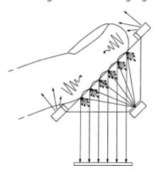
The LDE can block fake fingerprints made from paper, film, glue, rubber, clay and silicon all together by comparing images obtained with white lights and infrared rays.
