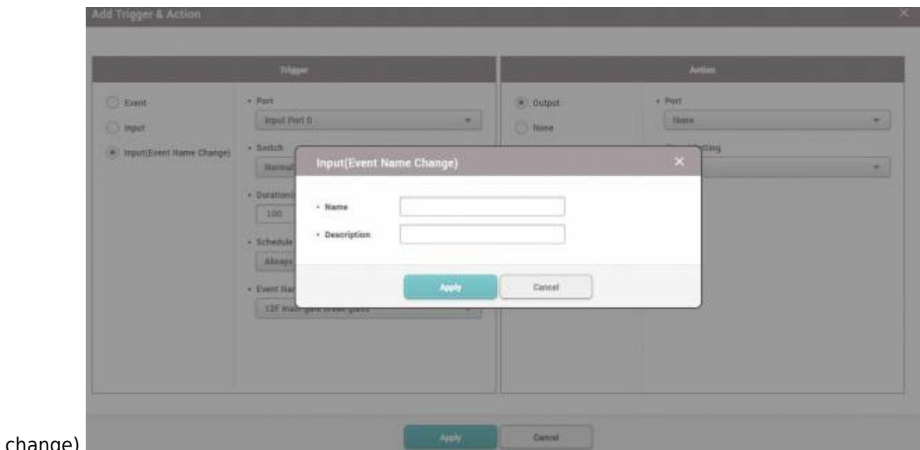
3. Choose 'None' for action when it does not need to output relay signals.
