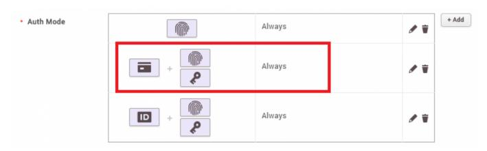
5-2. Once you succeed in card authentication on a 3rd-party device, the Wiegand input signal will be sent to the Suprema reader. After that, the Suprema reader requests you to scan fingerprints on it. If you succeeded in scanning fingerprints on the Suprema reader, the below event will happen as if "Card + Fingerprint" authentication is generated in one device.
