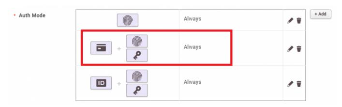
5-2. Once you succeed in card authentication on 3rd-party device, wiegand input signal will sent to Suprema reader. After that, Suprema reader requests you to scan fingerprint on it. If you succeeded in scanning fingerprint on Suprema reader, below event will happen as if "Card + Fingerprint" authentication is generated in one device.
