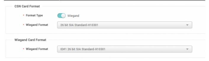
4. In the Advanced Setting, configure **Wiegand Input/Output** into **Input** and then select the suitable **In/Out Format**.
