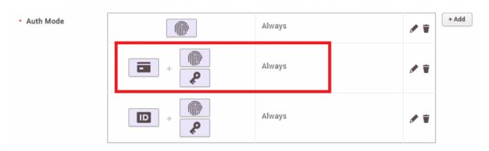
5-2. Once you succeed in card authentication on 3rd-party device, the Wiegand input signal will sent to Suprema reader. After that, Suprema reader requests you to scan fingerprints on it. If you succeeded in scanning fingerprints on the Suprema reader, below event will happen as if "Card + Fingerprint" authentication is generated in one device.
