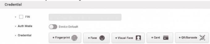
For the PIN, it's required to input four digits or higher numbers, and Auth Mode indicates whether you use private authentication mode for this user. And when you enroll fingerprints, make sure to start with the high-quality score(80 is recommended). This is because poor fingerprint quality can affect the matching performance.
