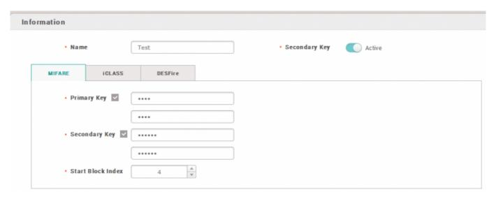
4) You can configure how many templates you want to store inside the card and which block to start on storing the information. You can also configure the template size, if you don't have enough space on the card to fit the template.
