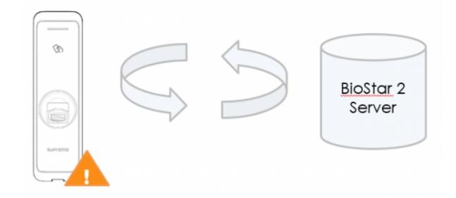
This means that the device has different access group, door, zone, and user information than the server.
