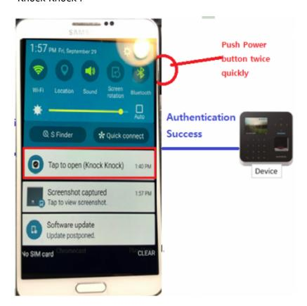
When BLE is connected, the smart phone vibrates shortly(200ms) first and it will vibrates longer(1000ms) when it communicates successfully. When communication is failed, it vibrates shortly again(200ms).
