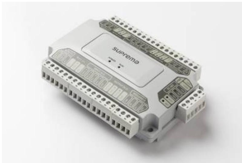
DM-20 is a door control module that controls Wiegand readers and various I/O devices. The DM-20 has 4 Supervised Input ports and various I/O interfaces. You can control the Wiegand reader's LED, Buzzer, Tamper, and more by engaging the DM-20 with BioStar 2.
