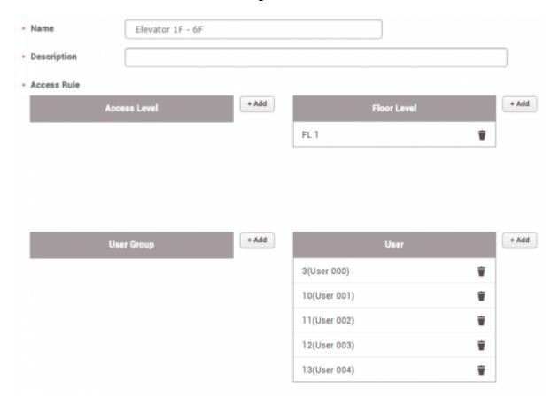
If configured like the image above, the buttons to access the 1st to 6th floor will be initiated for *User 000*, *User 001* and *User 002* when using *Elevator 1*.
