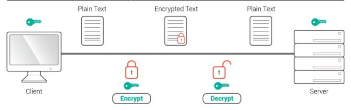
The size of symmetric keys are generally 128 or 256 bits and it is more difficult to crack passwords with larger keys. For example, the 128 bit key can have  $2^{128} = 340,282,366,920,938,463,463,374,607,431,768,211,456$  different combinations of passwords and it would take thousands of years in order to crack a 128 bit key with brute-force attack.
