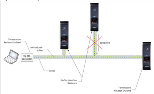
Do not use star-shaped wiring. This makes transmission line system complicated and hard to suppress line reflections if not impossible.
