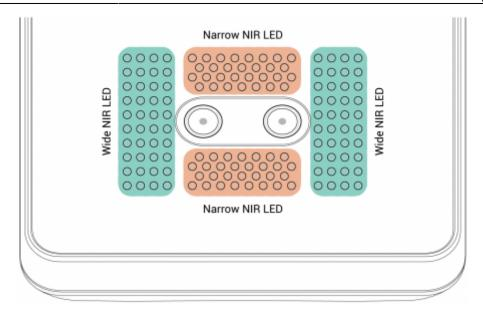
Another technology adopted by FaceStation 2 to enhance the performance is pixel intensity distribution analysis. One of the difficulties in using near infrared LED technology is the effects of ambient lighting. Ambient lighting can make near infrared LED lighting useless since it contains ultraviolet rays. Plus, the shadow on a face cast by ambient light can make it difficult for the face feature extraction algorithm to extract facial features.
