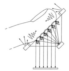
The LDE can block fake fingerprints made from paper, film, glue, rubber, clay and silicon all together by comparing images obtained with white lights and infrared rays.
