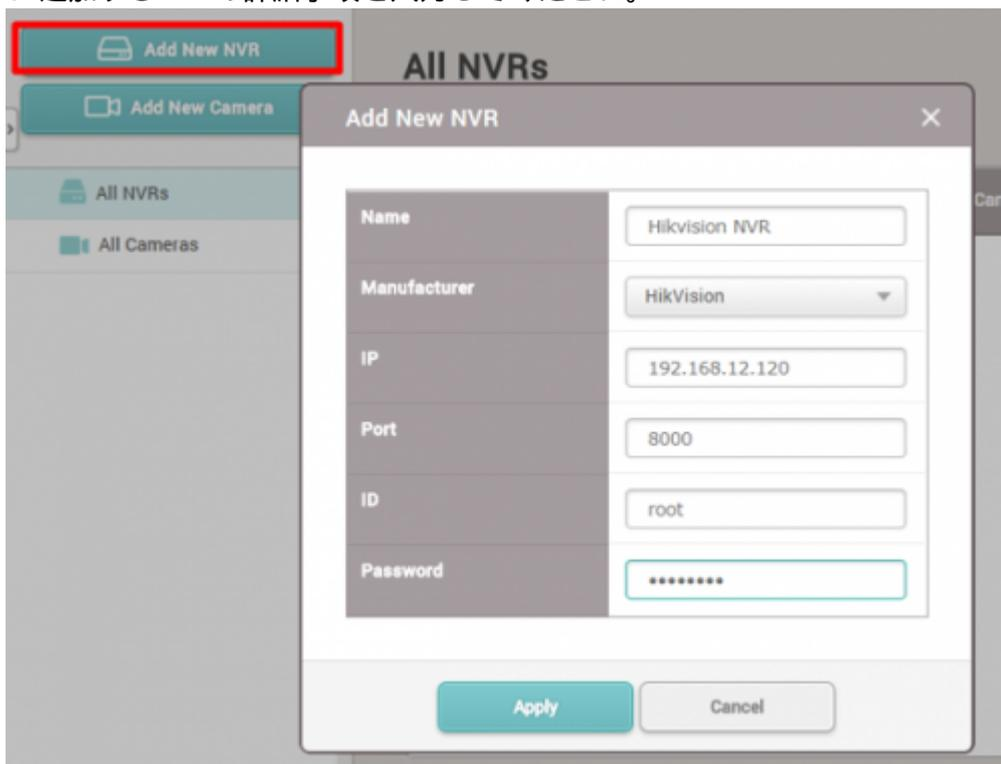
The screenshot shows the 'Add New NVR' dialog box in the BioStar 2 interface. The dialog box is titled 'Add New NVR' and contains the following fields: Name (Hikvision NVR), Manufacturer (HikVision), IP (192.168.12.120), Port (8000), ID (root), and Password (masked with asterisks). The 'Apply' button is highlighted in red.
