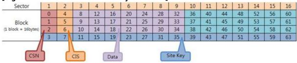
The MIFARE Classic 4K card has 40 sectors, 32 of which are divided into four blocks and the remaining 8 are divided into 16 blocks. 16 bytes (1 block) \* 4 blocks \* 32 sectors + 16 bytes (1 block) \* 16 blocks \* 8 sectors = 4096 bytes. The memory structure is as follows:
