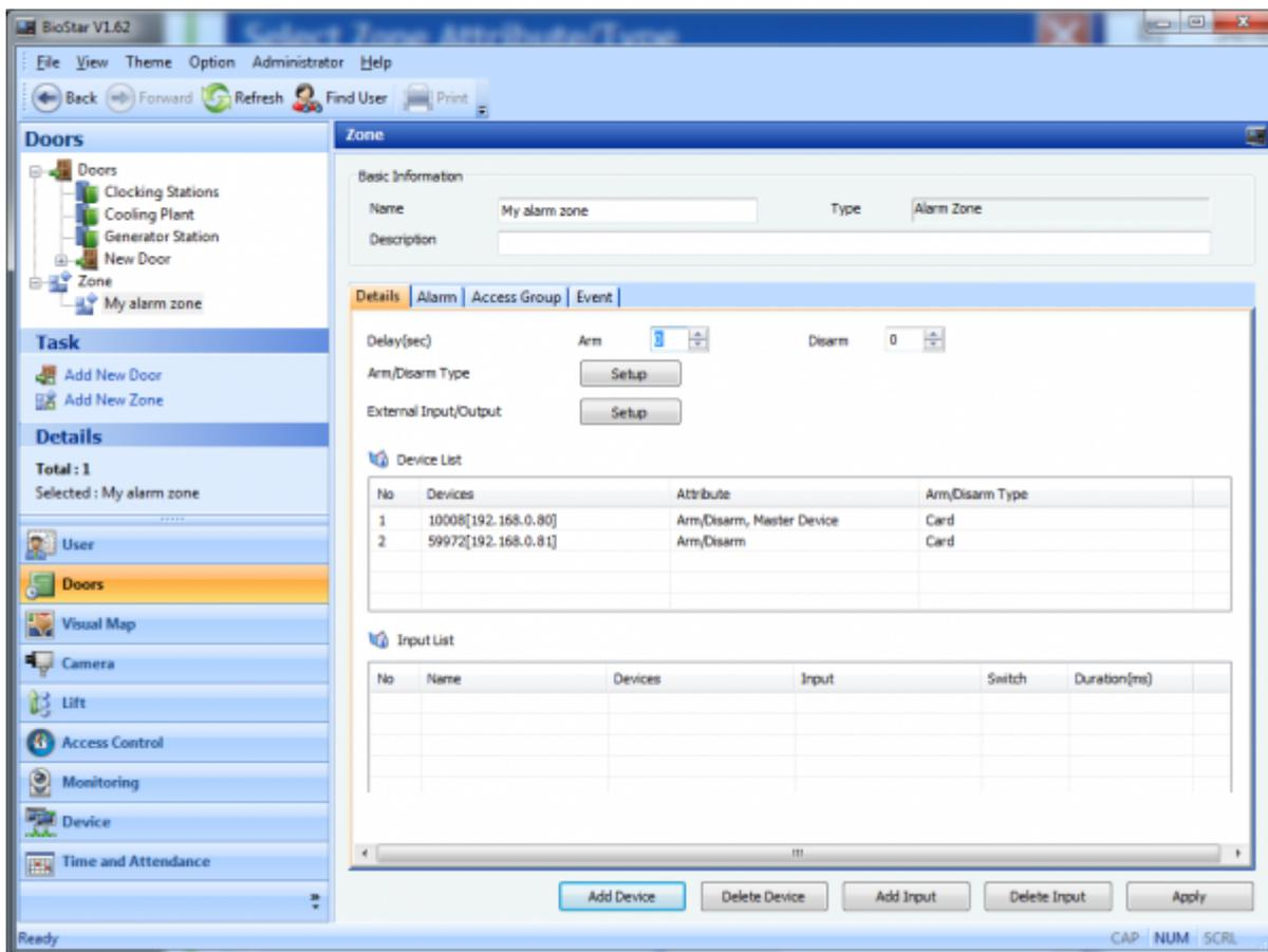
7. When there is an input signal from the input port specified here while the zone is armed, the alarm sets off.
