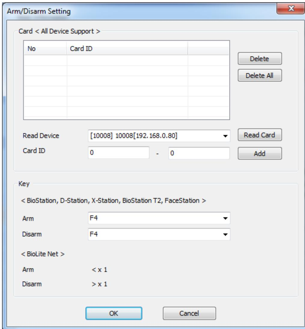
4) When we add the devices to this zone, we have chosen **Card** for the method to arm and disarm the zone, so the settings in the **Key** section on the dialog is not applied to this zone. If you have chosen **Key** for the **Arm/Disarm Type** option in step 5, you can arm and disarm the zone using the function keys of the device specified here.
