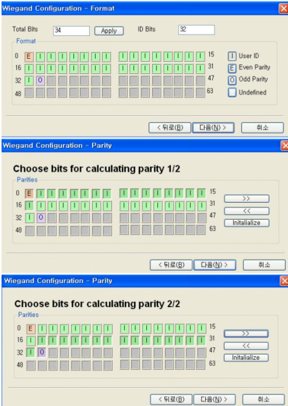
[Figure 12 Mifare Card Format Layout]
