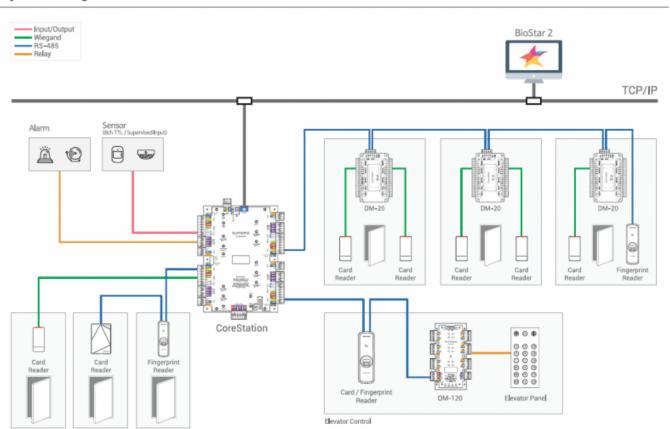
It can control multiple DM-20s with a daisy chain and also control multiple biometric device and card readers at once. The slave devices will be connected with a RS-485 connection and the 3rd party RF readers will be connected with Wiegand wiring.
