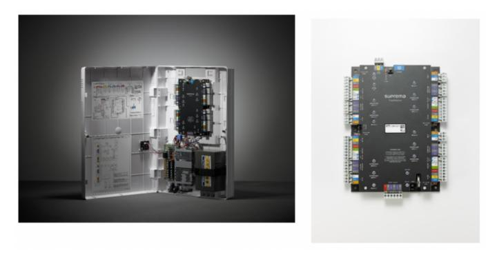
Since it is a centralized controller, CoreStation does not have a reading capability unlike other edge devices and its role is to control the slave and wiegand devices that are connected to the device. It has 4 relays, 4 wiegand inputs, and 5 RS485 channels where you can connect slave devices.
