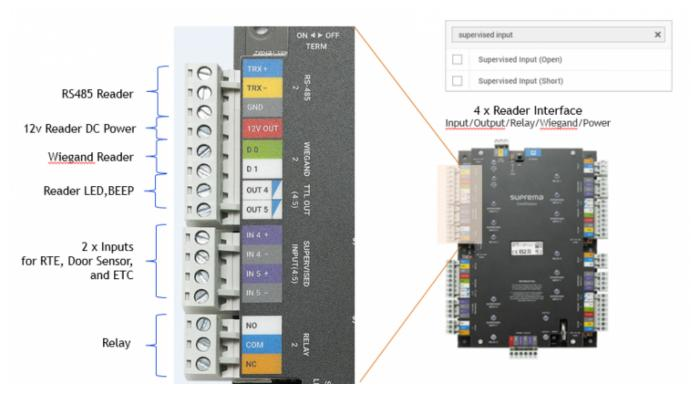
The device's input is supervised input. Which mean that the device can sense if the input has been tampered with just like the DM-20.
