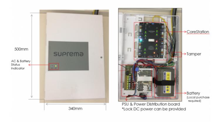
CoreStation also comes with an optional enclosure which includes the power supply unit and the power distribution board.
