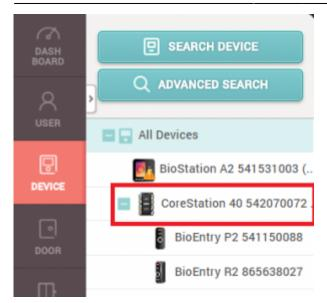
8. On **Advanced** configure your **Tamper** and **AC Fail** based on your wiring on the Aux Input to receive tamper and power failure logs.
