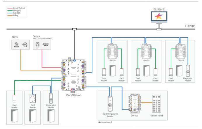
It can control multiple DM-20s with a daisy chain and also control multiple biometric device and card readers at once. The slave devices will be connected by a RS-485 connection and the 3rd party RF readers will be connected via Wiegand wiring.
