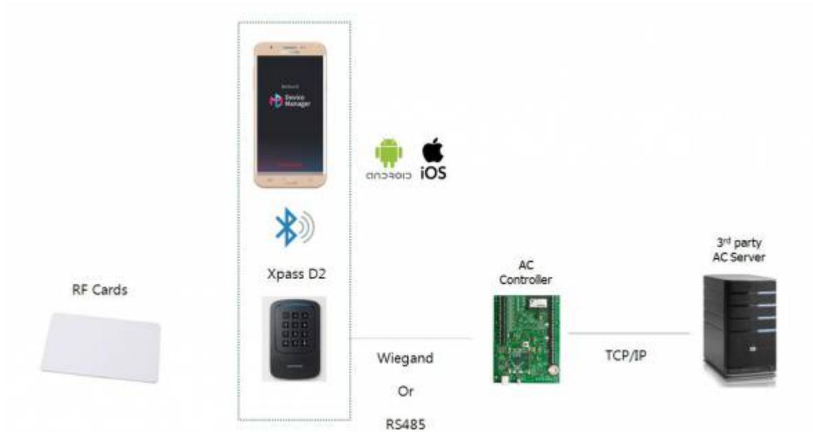
Device manager app can be used with XPass D2 FW 1.1.0 or higher. Manager app is compatible with all the XPass D2 models(MDB, GDB, and GKDB).
