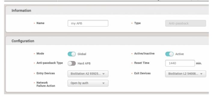
For a ethernet based zone, select **Global** for the **Mode**. The server will be the master device making anti-passback decisions.
