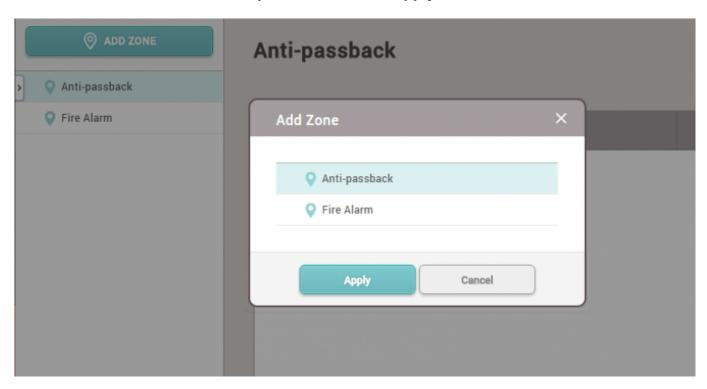
2. Enter the name of the APB zone, and make configuration as desired. If you want to block users who violate the APB rule, set the type to **Hard APB** and check **Reset Time** not to be shorter than the expected duration of the block time. And set **Entry Devices** and **Exit Devices**.
