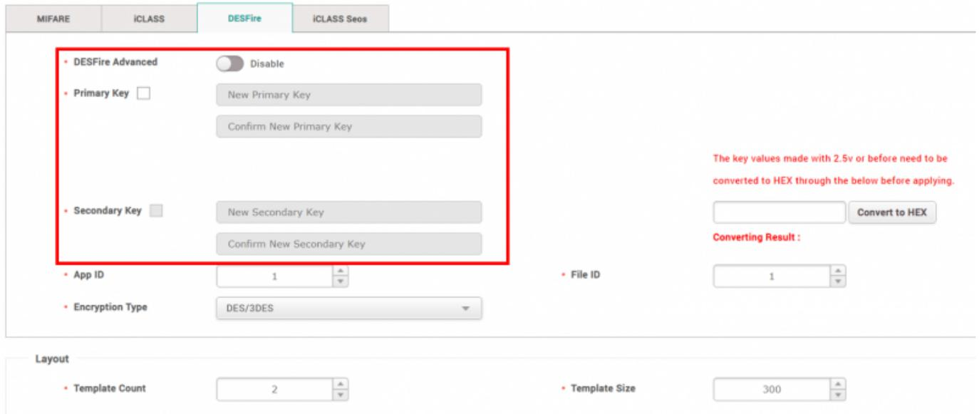
The screenshot shows the configuration interface for DESFire. The 'DESFire' tab is selected. A red box highlights the 'DESFire Advanced' section, which includes a 'Disable' toggle, 'Primary Key' and 'Secondary Key' input fields with 'New' and 'Confirm' buttons, and 'App ID' and 'Encryption Type' dropdowns. To the right, there is a 'Convert to HEX' button and a 'Converting Result' field. Below, the 'Layout' section shows 'Template Count' (2) and 'Template Size' (300).
